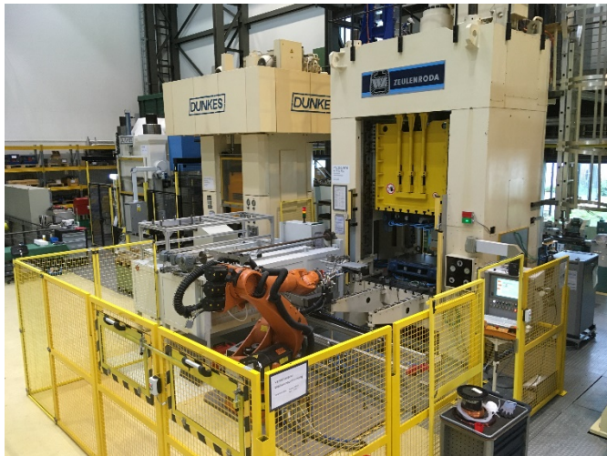
Fig. 1 Test rig for hot sheet metal forming at Fraunhofer IWU, including oven, press, and robot.
