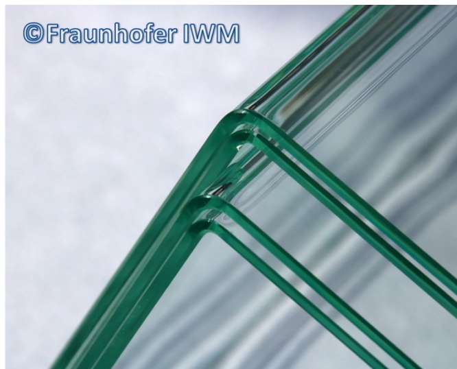
Fig. 2 The results of the glass-bending process: glass panes bent at a 90° degree angle.
