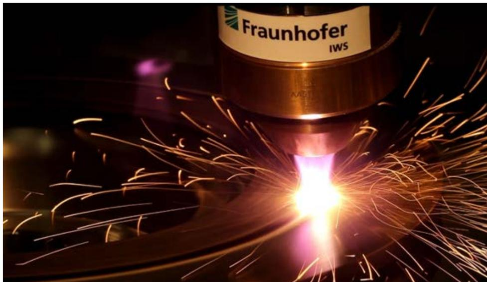
**HICLAD enables high-quality corrosion coatings in an efficient process.**
