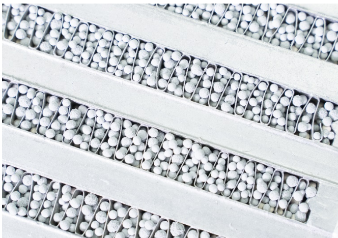
Picture 3 Heat exchanger with metallized zeolite.
