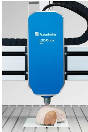
Picture 1: Thanks to the use of MEMS technology, the laser scanning microscope from the LSC-Onco project is so small and compact that it can be used to examine patients right on the operating table.
