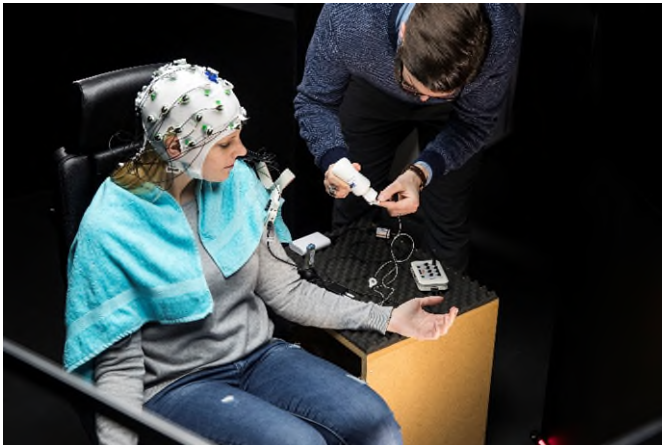
Fig. 2 Mathias Vukelic preparing for an EEG measurement and using gel to improve the conductivity of the electrodes.
