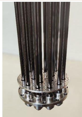
Fig. 2 The integrated membranes in the module for a reactor separate the hydrogen from the carbon dioxide.
