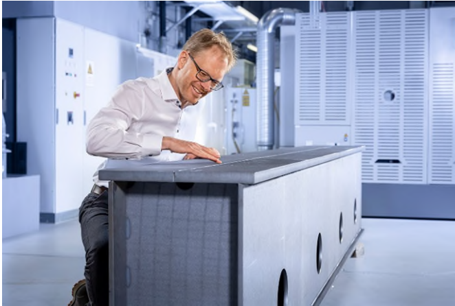
Fig. 1 Researchers at the Fraunhofer IWS used an indoor crane segment made of S355J2 structural steel (4 by 0.75 by 0.5 meters) to demonstrate that the laser MPNG welding process they had developed reduces energy costs by up to 80 percent and filler material consumption by up to 85 percent compared to conventional welding processes.
