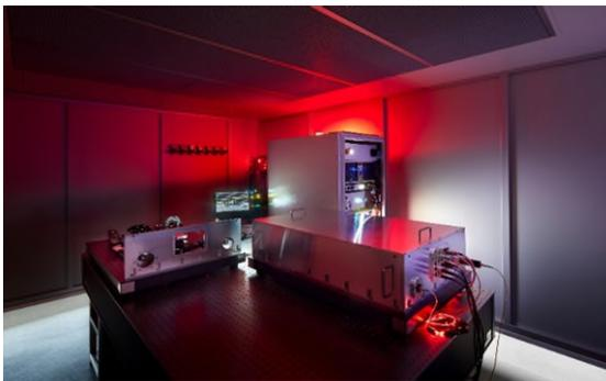
**Fig. 1** The quantum frequency converter developed by Fraunhofer ILT allows qubits to be transmitted with low noise and loss between distributed quantum computers via existing telecommunications networks.
