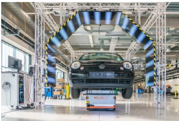
Picture 1: In the AutoInspect demonstrator, the car body is transported to the inspection stations on a conveyor system. The picture shows the deflectometry portal: The software can detect surface defects based on the reflection of the striped patterns displayed on the monitors.
