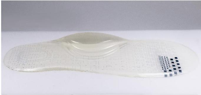
**Piezo sensors embedded in orthopedic inlays shall help analyzing the body balance and thus preventing posture problems.**
