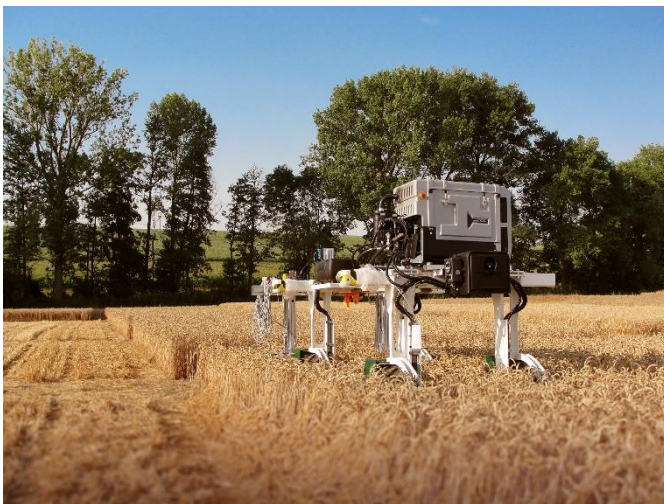
Fig. 1 The field robot DeBiFix examines whole wheat fields to show how the kernels are developing inside the ears. This can be used as a basis to determine which varieties are particularly suitable for breeding.
