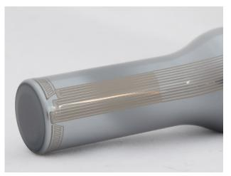
Sensor design with three temperature sensors and a structure for wear detection. © Fraunhofer IST, Ulrike Balhorn
