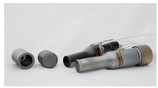
Two variants of a multisensory forming punch together with a blank and a pressed part. © Fraunhofer IST, Ulrike Balhorn
