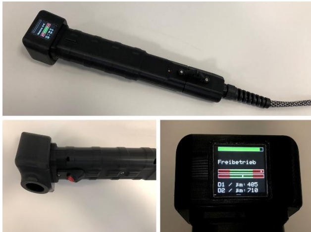
Fig. 3 The measuring head for the mobile terahertz system comes with a color display showing signal strength, operating mode and layer thickness results.
