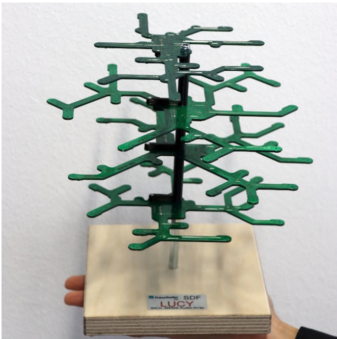
Fig. 2 The MEMS microphones are attached in a special geometric configuration in the array and can perceive sound from all directions. The array currently features 48 microphones, but this will increase to 256 in the future.
