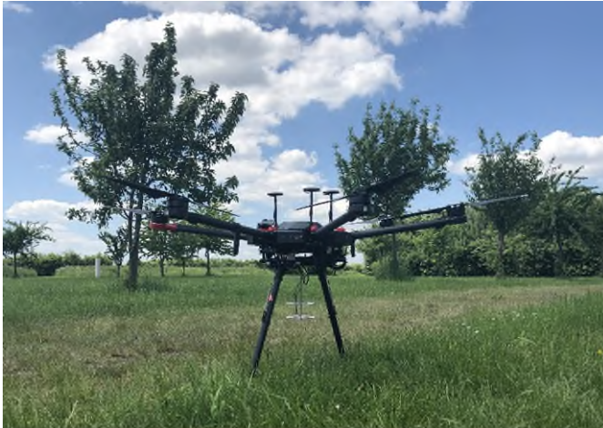
Fig. 3 The array of MEMS microphones — known as a crow's nest array — is mounted on a drone. It allows noises such as cries for help and knocking to be detected from the air and their direction to be determined.
