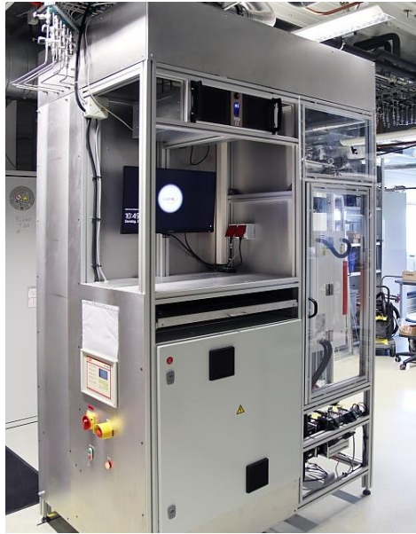
Figure 1: Direct reduction plant on a laboratory scale for reaction kinetic investigations and shaft furnace modeling.
