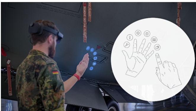
Fig. 4 Hand menu for controlling global system properties.
