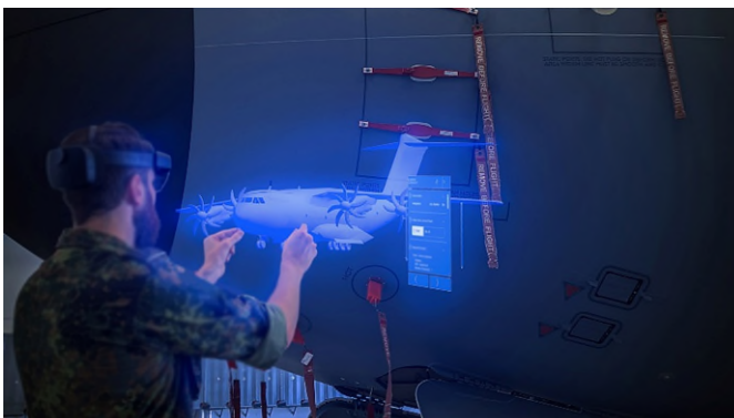
Fig. 1 Gesture control for scaling the 3D model of an aircraft.
