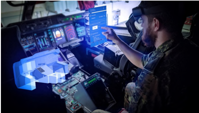
Fig. 2 Interaction with digital maintenance instructions for installing a display unit in the cockpit of an aircraft.
