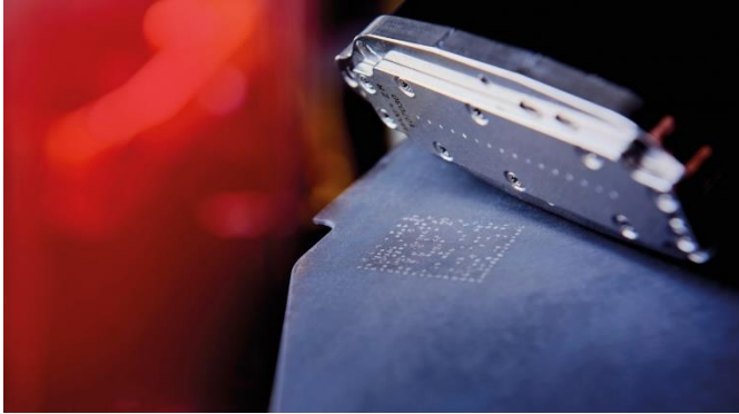
Picture 1: Data matrix code on hot-formed sheet metal, printed using industrial printer
