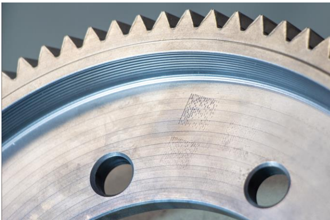
Picture 2: Printed data matrix code on a metal component
