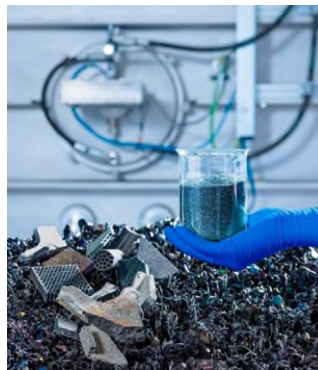
Fig. 1 RECOSiC ® uses waste and by-products from the Acheson process and turns them into high-purity silicon carbide in an enclosed high-tech furnace. The product of the process is powdered SiC.
