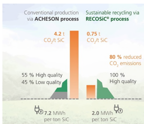
Fig. 2 The graphic depicts the advantages of RECOSiC ® compared to the Acheson process: CO 2 emissions and power consumption are lowered significantly, while the yield of high-quality SiC is much higher.
