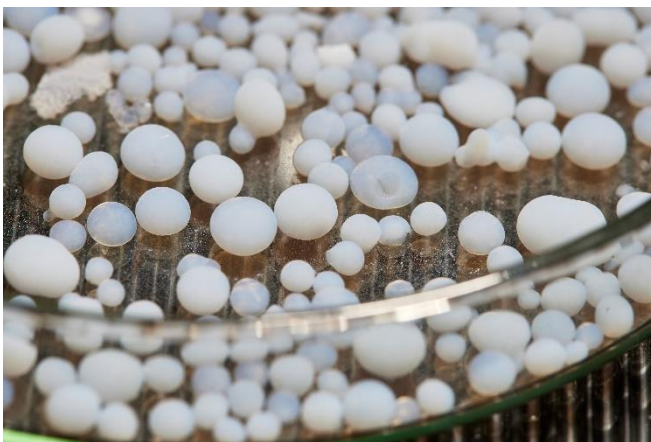
Fig. 2: The aerogel is broken down into grains 2 to 4 millimeters in size and mixed into insulation plaster.
