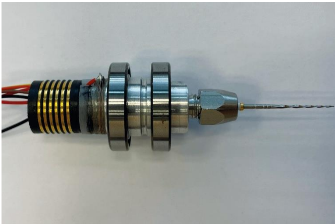
Picture 1: Dental file demonstrator with integrated piezoceramic stack actuator.
