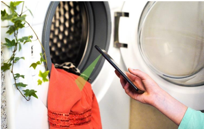
Fig. 1 If the label with cleaning instructions is no longer legible: A quick check with a smartphone, and the integrated spectrum analyzer recognizes the fabric the garment is made from. This allows you to set the correct wash cycle.
