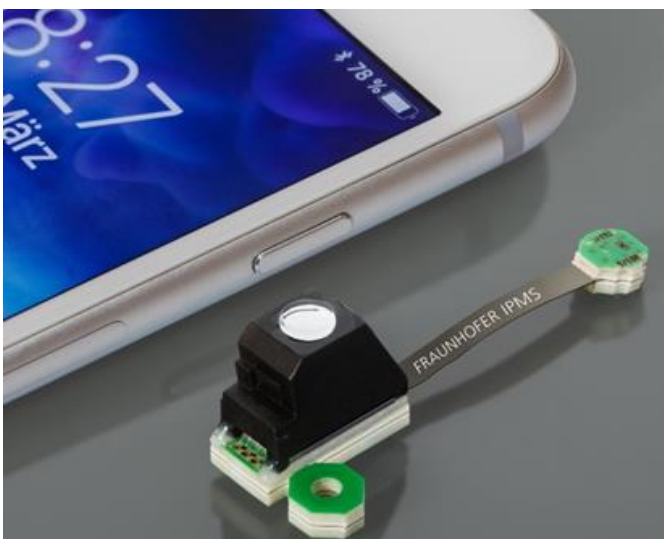
Fig. 2 The near-infrared spectrometer measures just 10 mm × 10 mm and is 6.5 mm thick. It fits into any standard smartphone. The system leverages the camera module for the analysis.
