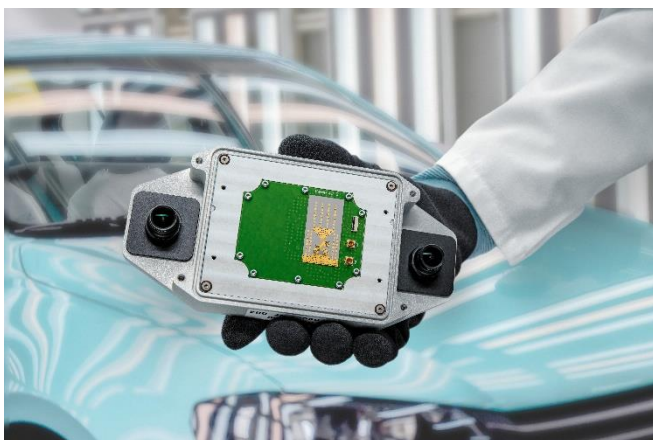
Fig. 2 Fraunhofer IZM's plug-and-play sensor platforms enable rapid testing and validation of concept ideas for wireless sensor and radar sensor systems.
