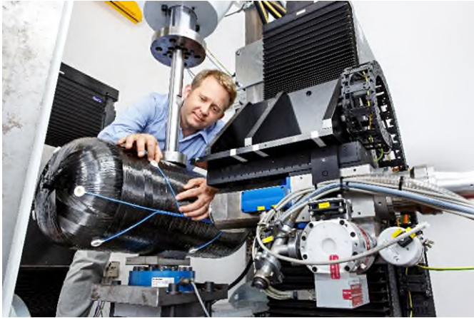
Fig. 1 The HyMon pressure tank is damaged before use at Fraunhofer LBF. The acoustic emission sensors detect damage to the tank and provide data for calculation models.
