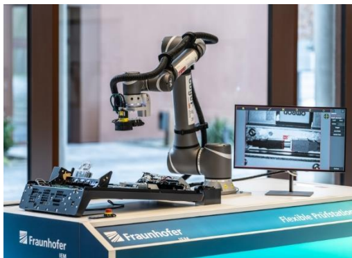
Fig. 2: The AI-powered image analysis software is integrated directly into the robot arm's camera module. If the software detects a defect, the system will notify the employees, who can then rectify the fault.
