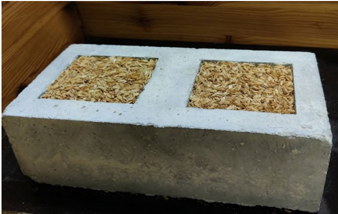
Fig. 1 Concrete component made of recycled aggregates and rice husk ash with rice straw insulation
