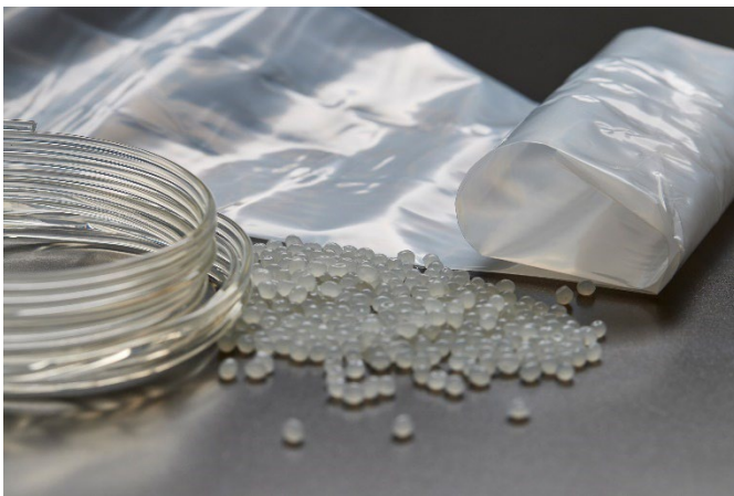
Fig. 2 The new PLA material can be processed into plastic films in a similar way to LDPE using conventional processing plants.
