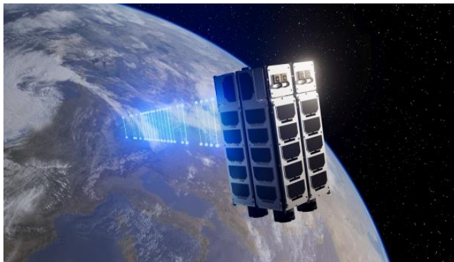
Picture 1: CubEniK project for ultra-secure encryption: The miniature satellite can transmit quantum keys over distances of 300 kilometers between two ground stations.
