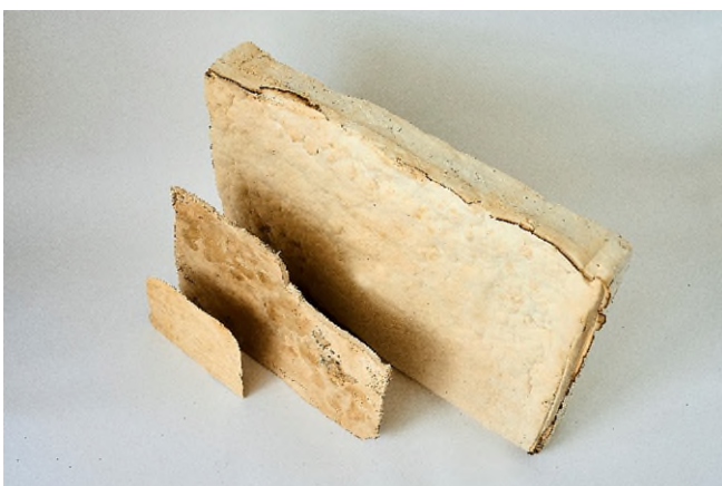
Fig. 2 Flexible mycelium materials in different thicknesses can be used as upholstery material, insulation board or alternatives to leather.
