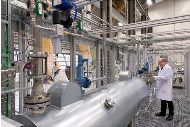
Fig. 1 Dr. Florian Mayer prepares to take measurements on the Bleed Air Contamination Simulator.
