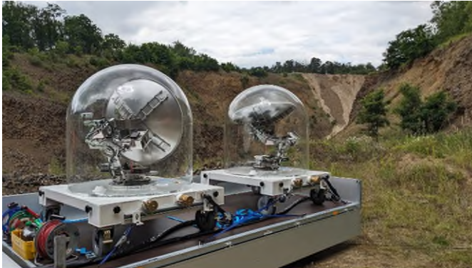
Fig. 1 Practical tests in a former basalt mine: The right-hand receiver antenna of the passive radar is aligned with a Starlink satellite, while the left-hand receiver antenna points toward the controlled landslide.
