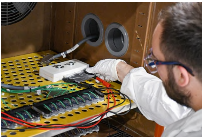
Fig. 2 Contacting a pouch cell with electrode materials from the ThüNaBsE project.
