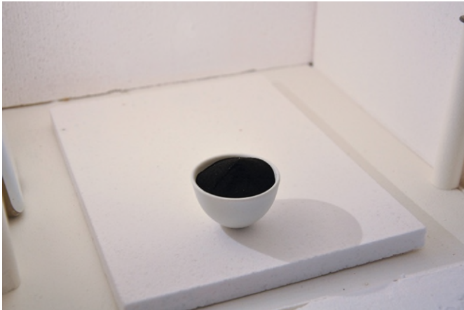
Fig. 1 Hard carbon, obtained from lignin, a by-product from the wood industry, forms the basis for the electrode of the Thuringian Forest battery.
