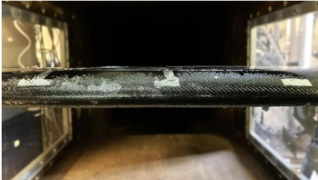
Fig. 2 Test in an icing wind tunnel: Realistic ice deposits form on the integrated leading edge of the wing.
