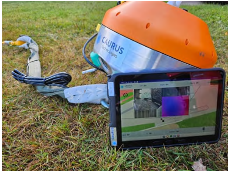
Fig. 1 The demonstrator shows how sensor data and simulations are combined to evaluate suppressant drops. © CAURUS Technologies
