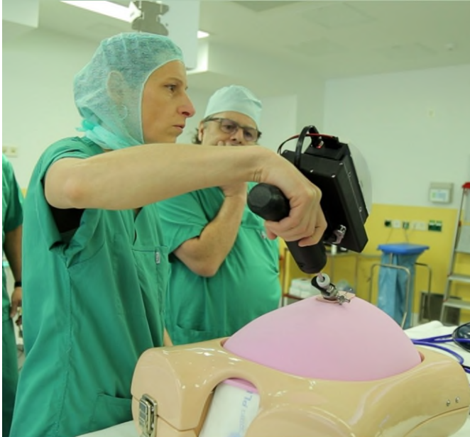
Fig. 1 The medical staff of St. Joseph Krankenhaus use an OR simulator to test the wireless endoscope prototype in an operating room. © Fraunhofer HHI
