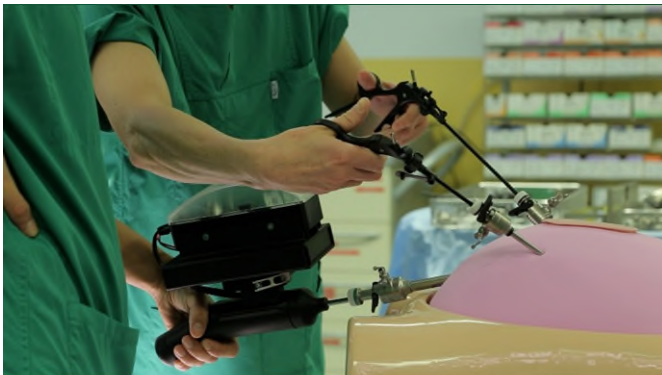
Fig. 2 Optical wireless communication (LiFi) ensures robust data transfer from the endoscope to the monitor even under adverse conditions. © Fraunhofer HHI
