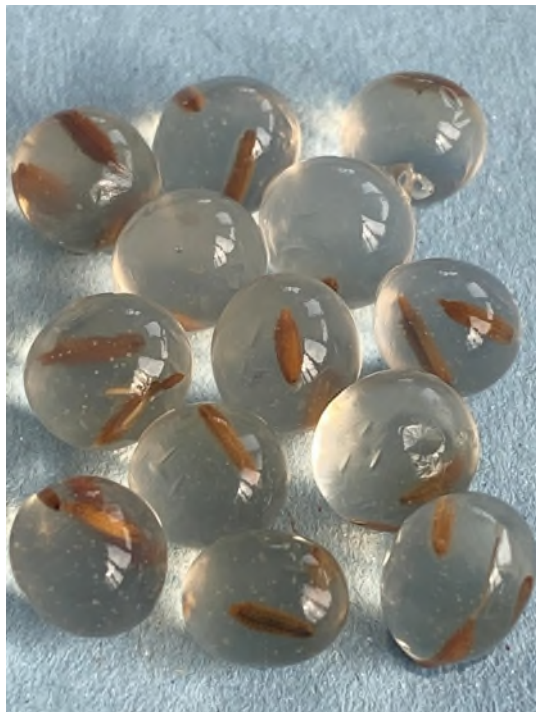
Fig. 2 Dandelion seeds in alginate capsules produced using the dripping process © Fraunhofer ICT
