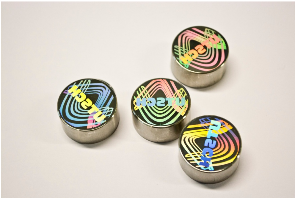
DLIP-generated exemplary product protection feature
