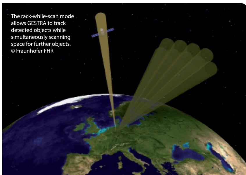
the beams — or “lobes” as we call them — you can not only scan large areas very quickly and flexibly for objects but also set aside one lobe for object tracking, while the remainder continue searching independently of the tracking lobe. This track-while-scan mode is optimized for use in space surveillance,” explains Ben Bekhti.
