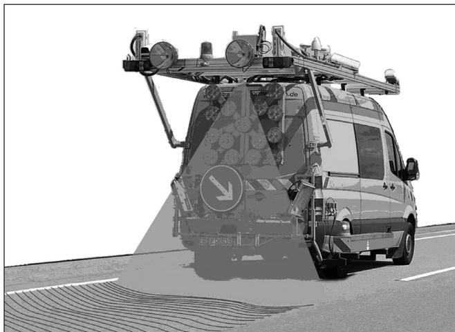
**A single laser scanner is all it takes to measure the evenness of a road four meters in breadth with a laser beam.**
