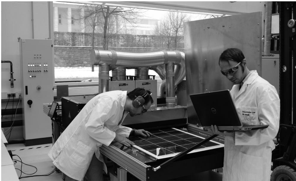
Scientists are laminating a solar cell at CSP in Halle. The process is twice as fast as it used to be.
