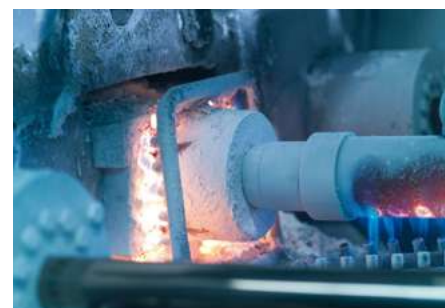
Gas-powered magnesium pressure casting process: a starting point for bivalent energy supply.
