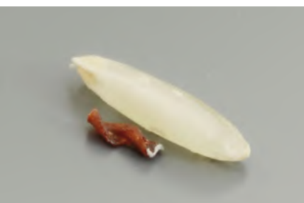
The micro-robot is 3 millimeters long and 1.2 millimeters in diameter — that is smaller than a grain of rice.
