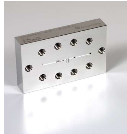
The FDmiX mixer: simple and precise production of nanoparticle shells for mRNA therapeutics
