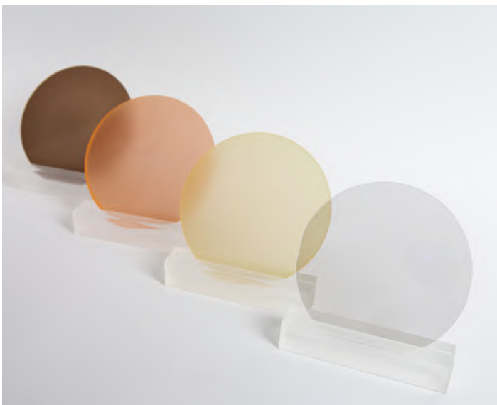
The production of AlYN/GaN wafers using the MOCVD process, which can be seen here in various yttrium concentrations, is a breakthrough in the field of semiconductor materials
