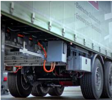
Autonomous electric drive collaboration system for truck and vehicle trailers Image: evTrailer Zeichnung/ CuroCon GmbH
