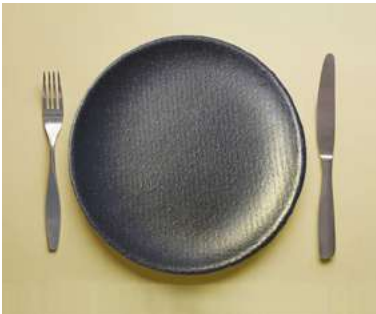
▲ This plate was produced during pilot trials using a film made of sugar beet pulp Photo: Fraunhofer WKI
