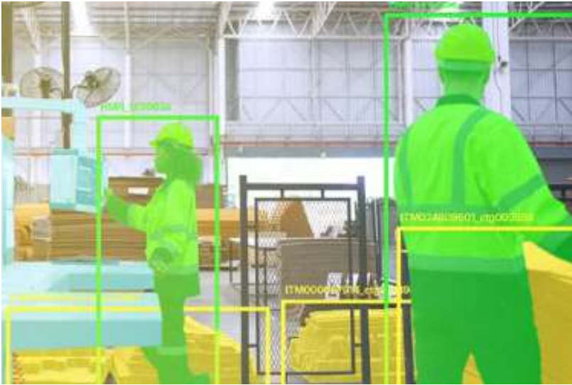
▲ Reliable person detection for safe cooperation between humans and robots Photo: Fraunhofer IKS
