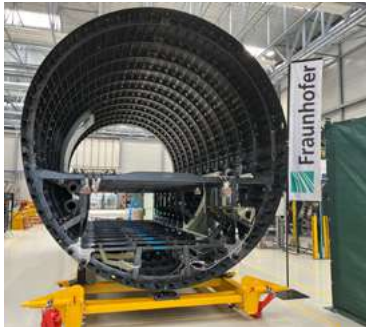
The aircraft fuselage section at Fraunhofer in Stade, fully joined by thermoplastic welding Photo: Fraunhofer IFAM
