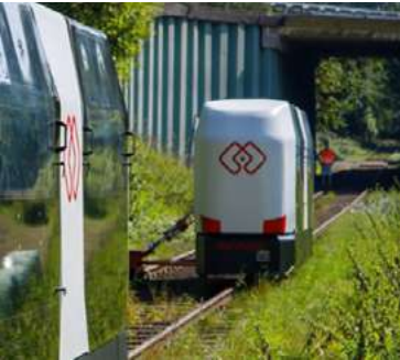
Self-driving monorail vehicle on the test track in Extetal Photo: MONOCAB
